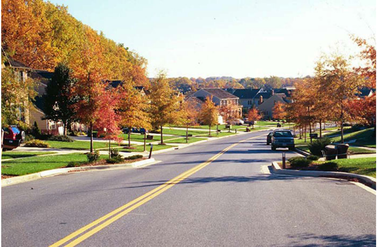
Figure 3.17.4. Choker in Suburban Residential Setting
