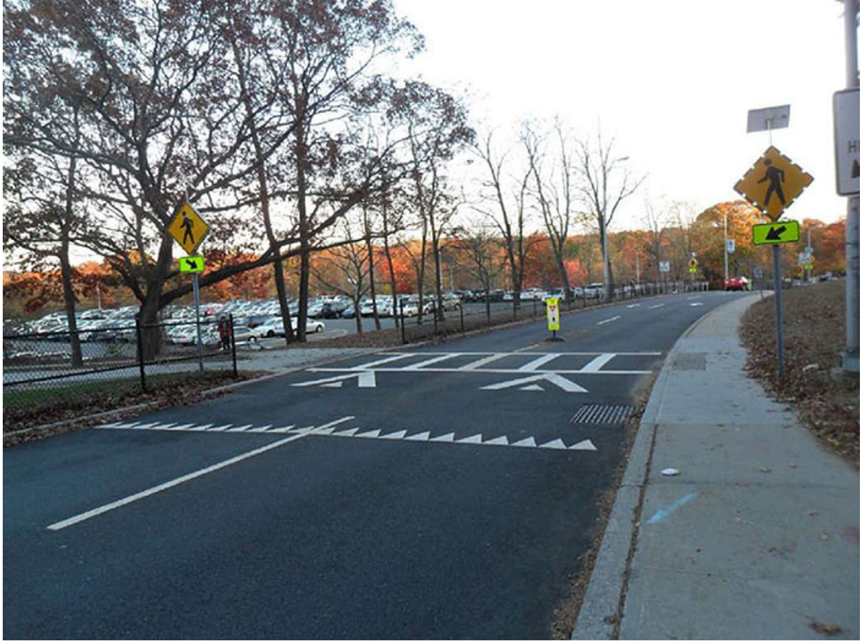
Figure 3.14.3. Raised Crosswalk Midblock
